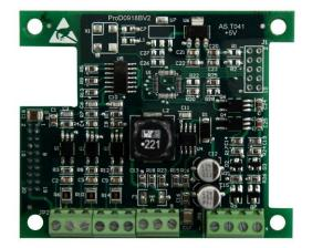
Fig 4.23 ABZ incremental 5V PG card terminal layout
