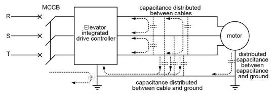
Figure A5.1 Paths of Leakage Current
