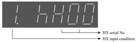
The above figure show: HX0 has no input. Press up or down to select HX serial No. serial no start from 0-15. after finishing the selection of corresponding serial no HX, the figure in the highest order show the input to this input terminal is valid or not ( o represent no valid input , 1 represent
