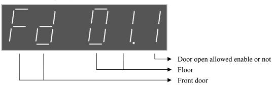
The above picture mean: shield 1 floor front door open allowed. Fd is the abbreviation of Front door. Press the up and down button to browse the front door open allowed parameter of corresponding floor. Press the enter button to make modification. The figure in the lowest order starts to flash, use up or down button to modify the figure into 0 or 1. Press the enter button to confirm the modification (0 is to shield front door open allowed function, 1 is to allow front door open function)
