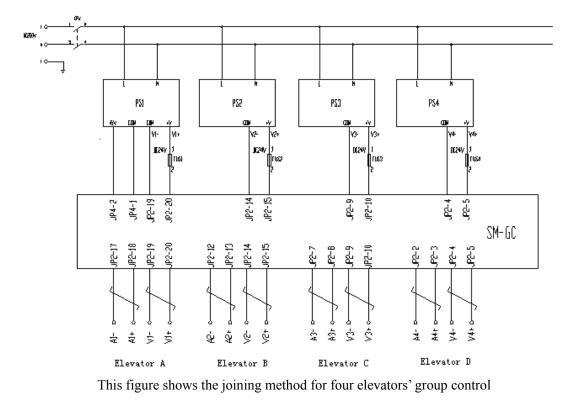
PS1, PS2, PS3, PS4 are switch power supply, PS1 has +5V (3A) and +24V (1.8A) output, PS2, PS8 and PS4 have only +24V(1.8A) output. FU1, FU2, FU3, FU4 are over-current protection devices, SM-GC is group control board.
