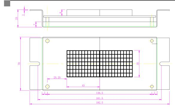
Fig. 6.18 Mounting Dimensions of SM-04-HSC
