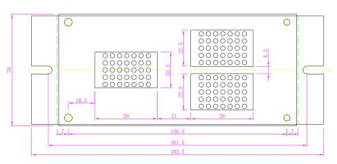
Fig 6.12 SM-04-VRF installation dimension
