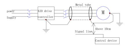
Fig 4.15 the wiring arrangement schematic diagram of main circuit
