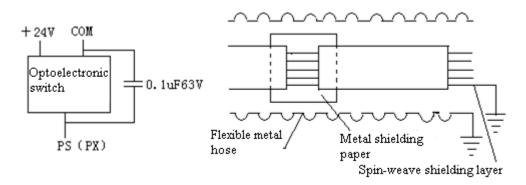
Figure 8.6 Capacitor connection diagram
