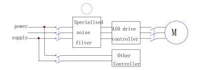
Fig 4.7 the right setting of noise filter at the side of power supply The wrong setting of noise filter at the side of power supply is as fig 4.8 and fig 4.9
