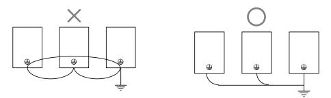
Fig 4.5 multi-elevator integrated drive controllers wiring
