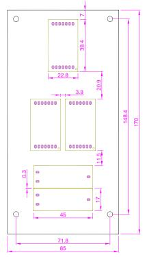
Fig 6.30 SM-04-VRJ installation dimension
