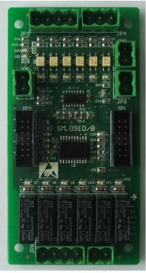
Fig 6.3 car top extension board outside view
