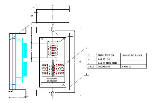
Fig. 6.20 Mounting Dimensions of SM-04-VHL
