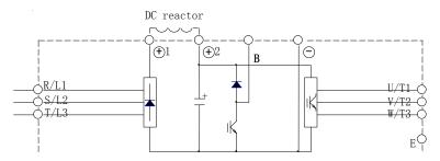
Fig 4.11 external connected DC reactor wiring
