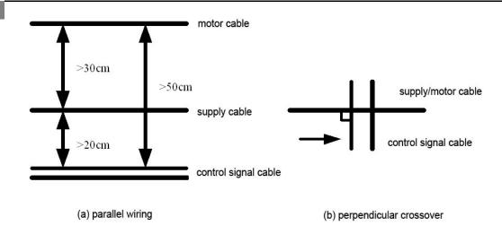
Figure A2.1 Requirements on cable laying
