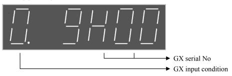
The above figure show the GX0 has no input, press up or down to select GX serial no the serial no start from 0 to 15. After finished the selection of corresponding serial no GX, the figure in the highest order show the input to this input terminal is valid or not. (O represents no valid input. 1 represent valid input)
