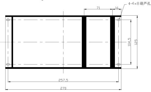
Fig 6.9 instruction controller board installation dimension
