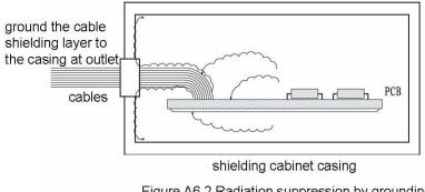
Figure A6.2 Radiation suppression by grounding the cable shielding layer to the casing
