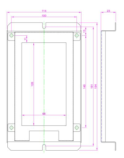
Fig 6.26 SM-04-VL/B3 installation dimension Table 6.16B SM-04-VL/B3 plug-in specification and port definition
