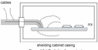
Figure A6.1 Radiation from output cables from shielding cabinet
