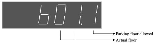
Use up and down button to select the floor need to modify. Please note, the floor mentioned here is the actual floor ( or the control floor) press the enter button. The selected value start to flash, press the up and down button to set the value. press the enter button to confirm, in which 1 mean parking allowed, 0 mean parking prohibited.
