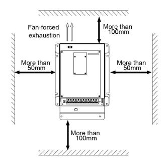
Figure 2.2 Requirements on Installation Clearance
