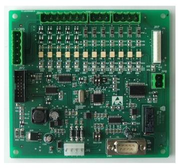
Fig 6.1 car top control panel outside view
