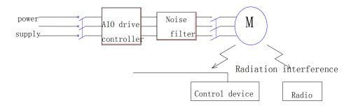
Fig .4.14 the wiring at the output side of integrated drive controller
