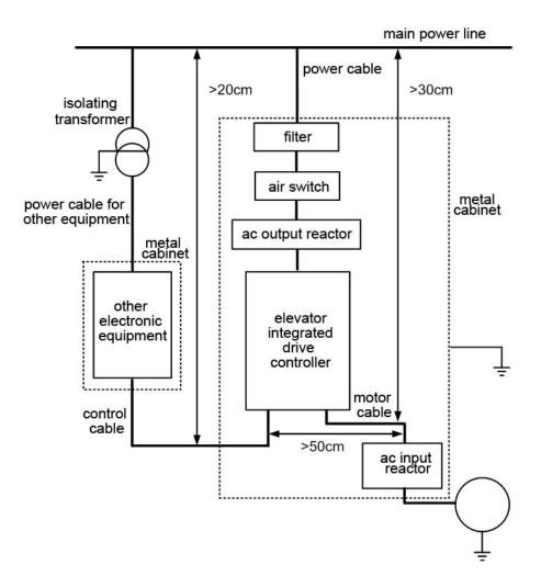
Figure A9.1 Electric Installation of elevator integrated drive controller In order to meet the EMC directive, the following notices must be taken:
