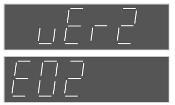
The menu shows the program version of control part of integrated unit. The screen will display the program version E02 of the control part one second later, as per the above picture. Then the words VER 2and E02 will alternatively display, each of which will last for 1 second.
