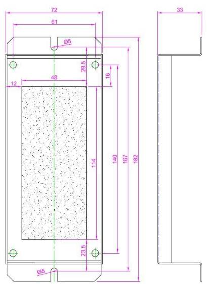
Fig.6.24 Mounting Dimensions of SM-04-VL16/A
