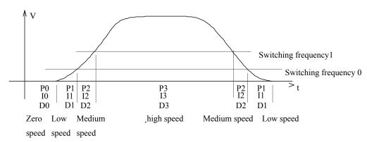
Diagram 8.3 Elevator operation curve segment PI control chart
