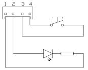
Fig 6.7 door opening/closing button and instruction lamp connection diagram
