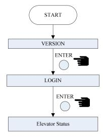
Picture 5.5 operations from power on to elevator status window
