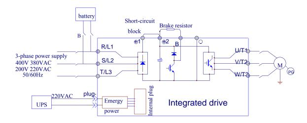
Fig 4.6 schematic diagram of emergency power supply and battery wiring
