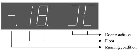
This menu will display the basic condition of elevator, including running condition, floor located, and door condition.
