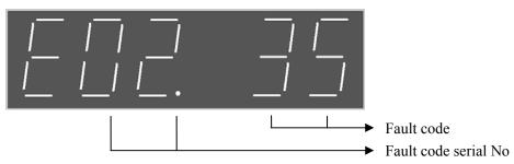
The integrated unit can save up to 20 fault code. The latest fault code serial no is 00. use up or down key to browse the these fault code. Press enter key to display the fault date, press left or right key to check the time and floor that fault occurred. Press esc to quit.
