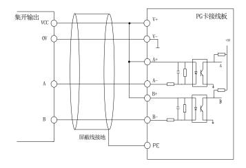
Fig 4.20 the wiring of encoder push-pull signal
