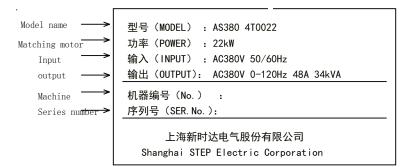
Fig 1.2 Nameplate description of elevator integrated drive controller 1.5 Notice Items for safety
