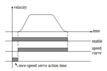
Figure 8.1 Zero Servo Timing Sequence Diagram
