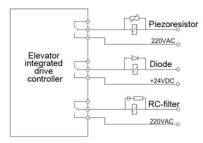
Figure 4.1 Use Requirements of Relay, Contactor and Electromagnetic Brake
