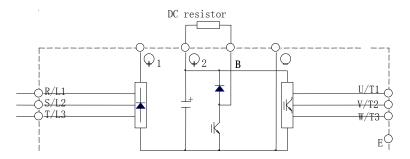
4.4.5.6 elevator integrated drive controller output terminal (U/T1, V/T2, W/T3)
