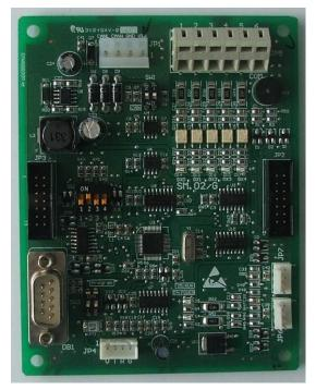
Fig 6.5 car controller outside view
