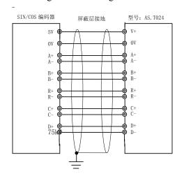
Fig 4.2.2 the wiring of sin/cos differential output signal of encoder
