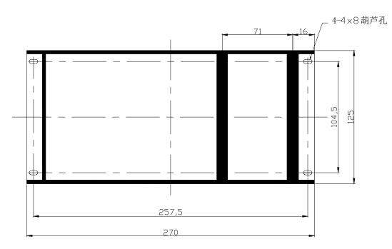
Fig 6.5 car control panel installation dimension
