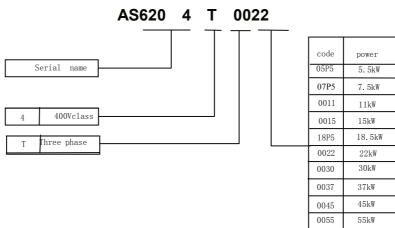
Fig-.1.1 Description of inverter type
