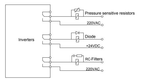
Fig- A.7Operation requirements on relays, contactors and EM brakes
