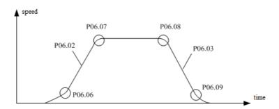
Fig-7-7 S curve by's position during motor running
