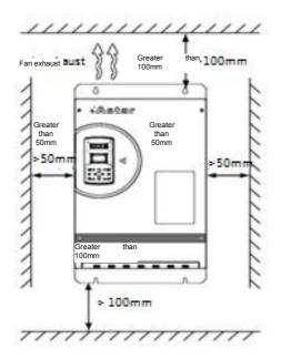
Fig-. 3.1 Schematic of spacing of inverter installation
