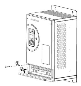
Fig-. 3.5 Opening wiring cap
