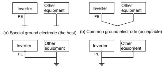
(c) Common ground electrode (unacceptable) (d) Common ground electrode (unacceptable)
