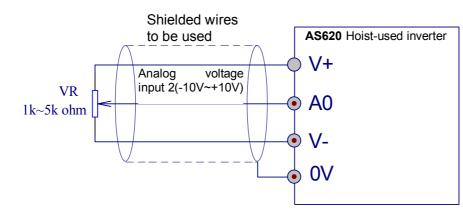
Fig- 4.18 Analog input signal shielded wire wiring
