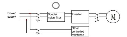
Fig- 4.7 Noise filter on the power supply side
