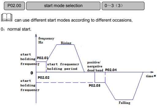
Fig- 7-1 start frequency start mode diagram
