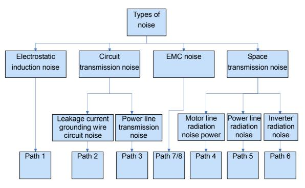
Fig-A.1 Schematic of the types of noise
