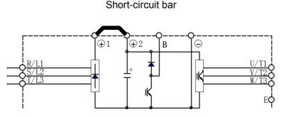
Fig- 4.10 Wiring diagram of short-circuit bar
