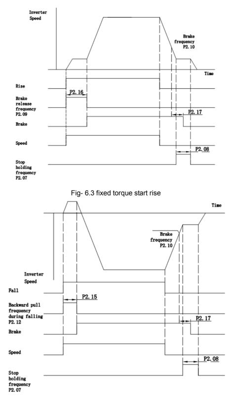
Fig- 6.4 fixed torque start fall
