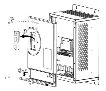
Fig-. 3.6 Removal of front panel
