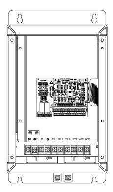
Fig-. 4.2 Internal view of inverter
