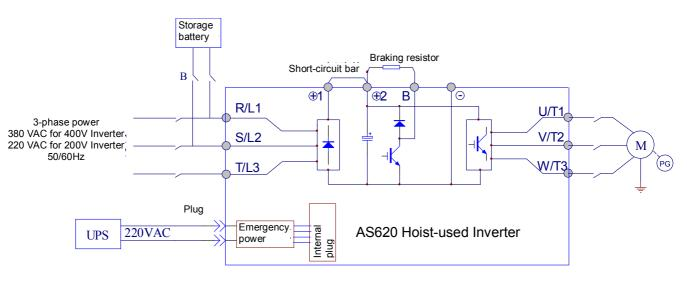
Fig- 4.6 Emergency power and storage battery connection
