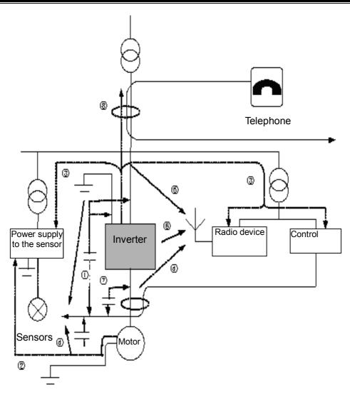
Fig-A.2 Noise transmission schematic
