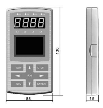
Fig-. 2.2 Dimension of inverter's operating device
