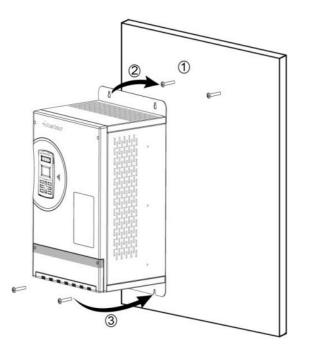
Fig-. 3.2 Diagram of inverter installation order
