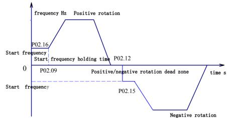
Fig- 7-2 positive/negative start frequency start mode diagram
