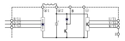
Fig- 4.11 Wiring of the external DC reactor
