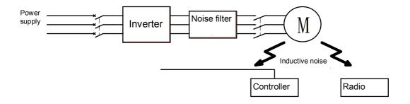
Fig- 4.14 Connection of noise filter on the output side of the Inverter
