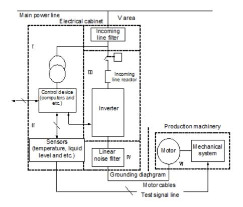
Fig-A.11 Schematic of installation area for the inverter's EMC
