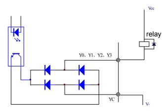
Fig- 4.20 Circuit of open collector ouputs
