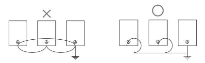
Fig- 4.5 Grounding method of more than one Inverter
