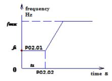
Fig- 7-3 start frequency and start time diagram
