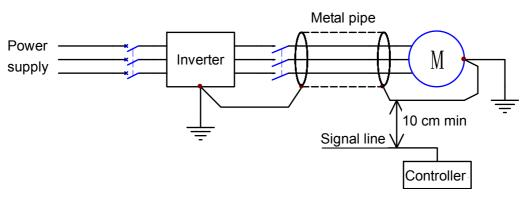
Fig- 4.15 Main circuit wiring
