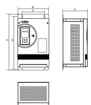
Fig-. 2.1 Installation dimension and quality of inverter
