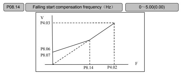
Fig- 7-9 falling start compensation frequency diagram
