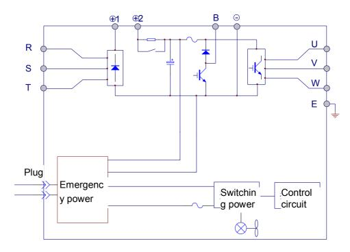
Fig- 4.4 Main circuit conFig-urations
