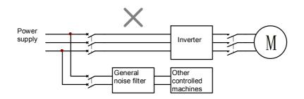
Fig- 4.9 Example 2 of incorrect noise filter setting on the power supply side
