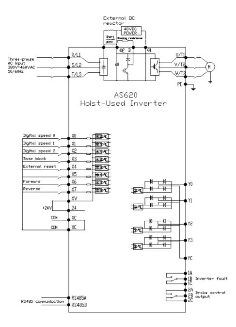
Fig-. 4.3 Wiring diagram of inverter terminals
