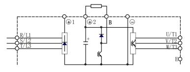
Fig- 4.12 External braking resistor wiring
