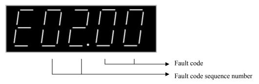
CD/A can store 20 fault codes. The nearest fault code sequence number is 00. Use the "up" and "down" buttons to browse these fault codes.
