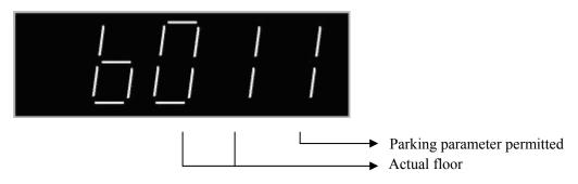
Use the "up" and "down "buttons to select the floor to be modified, please take notice that the floor herein is actual floor (or control floor).Press "Enter", the parameter begins to flash, use the "up" and "down" buttons to set the parameter, then press "Enter" again to affirm, where the "1"denotes permitting to park, "0"denotes forbidding to park.
