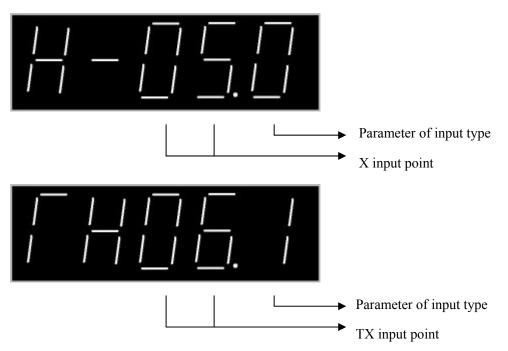
Use the "up" and "down" buttons to select X or TX input points to be modified. Press "Enter", the parameter begins to flash, use the "up" and "down " buttons to set the parameter, then press "Enter" again to affirm, wherein the "1"denotes normally closed contact, "0"denotes normally opened contact. Notes: due to the limit of seven segment code, the "T" and "X" in CD/A are all as the figure above, wherein the showing "X" is similar to "H", do not mistake it.
