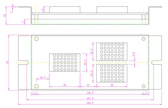
Fig. 2-7 (B) Mounting Dimensions of SM-04-VRF
