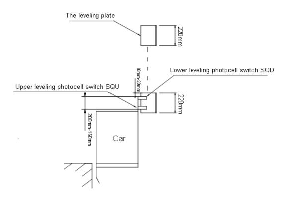
③ The leveling plates of every floor should be in alignment with the inductor by the central line for better leveling performance after recording the floors.
