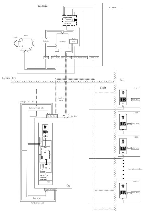
Fig. 2-1 Configuration of Serial Control System
