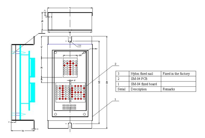
Fig. 2-11 (B) Mounting Dimensions of SM-04-VHL
