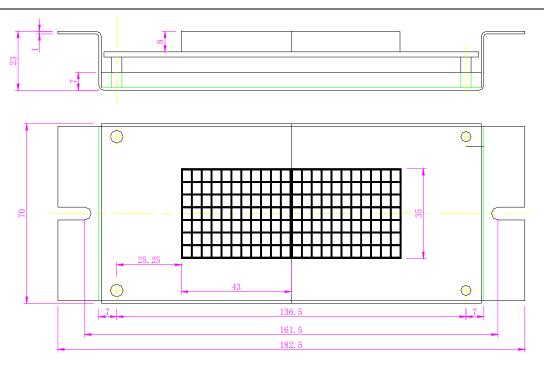
Fig. 2-10 (B) Mounting Dimensions of SM-04-HSC
