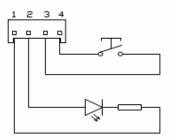
Fig. 2-4 Connection of Door Open/Close Buttons & Indicators
