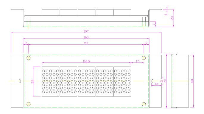
Fig. 2-9 (B) Mounting Dimensions of SM-04-HRC
