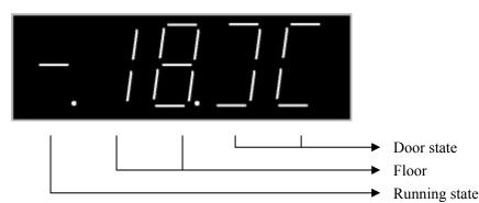
In this menu, you can see the basic states of elevator, including running state, current floor and door state. During the running state:
