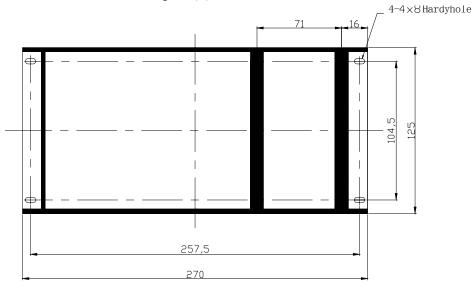
Fig. 2-3 (B) Mounting Dimensions of Car Board
