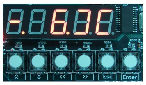
Figure I.1 LED, press-button drawing of partial enlargement
