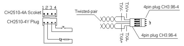
Fig. 2-13 (A) Connection of the Push Button
