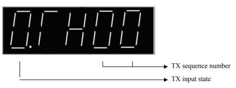
The meaning of figure above is that TX0 shows having no input. Use the "up" and "down" buttons to select TX sequence number whose range is from 0 to 23. After selecting the TX sequence number, the highest order indicates whether having the valid input at the input terminal or not (zero denotes having no valid input, while one denotes having valid input).
