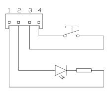
Fig. 2-6 Connection of Door Open/Close Buttons & Indicators
