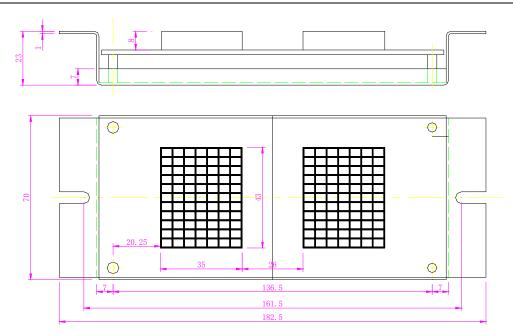
Fig. 2-8 (B) Mounting Dimensions of SM-04-VSC
