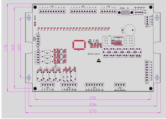
Fig. 2-2 (B) Mounting Dimensions of Master Control Board
