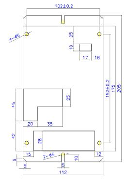
Fig. 2-12 (B) Mounting Dimensions of SM-04-UL
